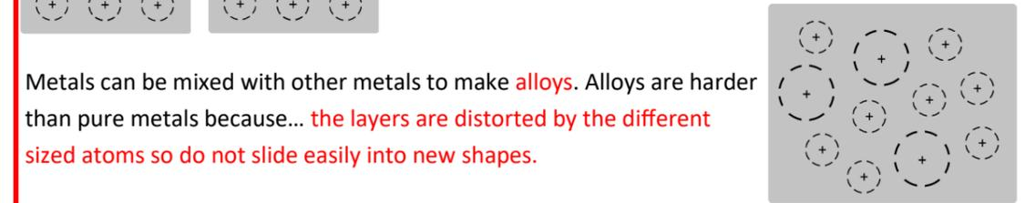
Metals can be mixed with other metals to make **alloys**. Alloys are harder than pure metals because... **the layers are distorted by the different sized atoms so do not slide easily into new shapes.**
