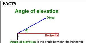
Angle of elevation is the angle between the horizontal and a line in a direction above the horizontal.
