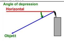
Angle of depression is the angle between the horizontal and a line in a direction below the horizontal.
