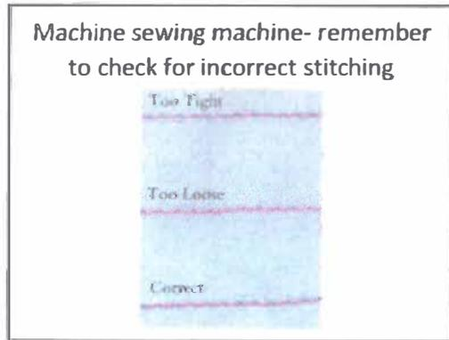
Machine sewing machine- remember to check for incorrect stitching
